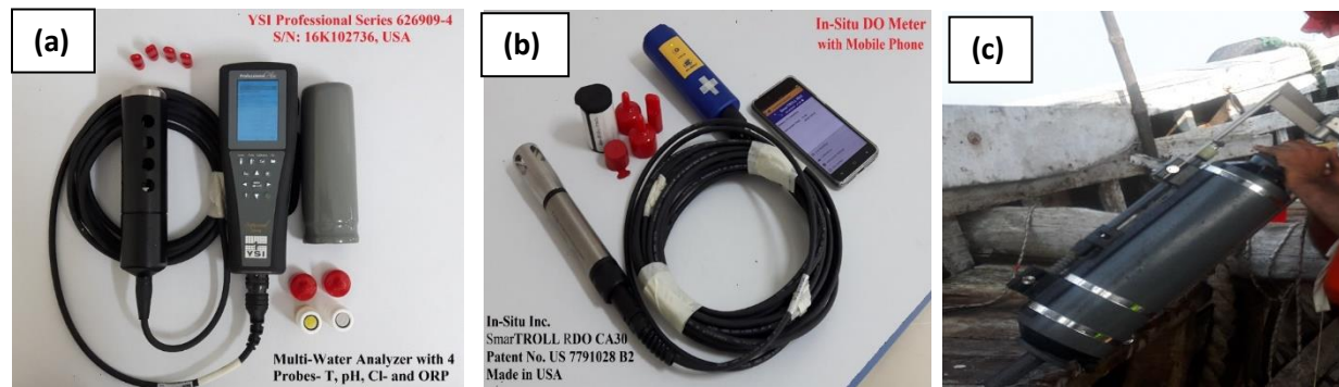
Fig. 2. (a) Multi-water analyzer (YSI Professional Series-626909-4, Made in USA), (b) In-Situ DO meter (SmarTROLL RDO CA30, Made in USA) and (c) Niskin Water Sampler
